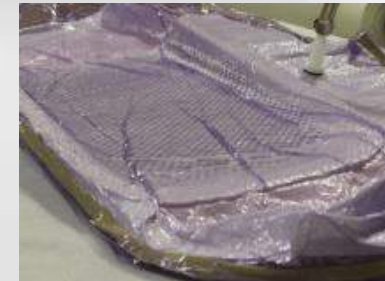
Vacuum bagging of prepreg lay-up
