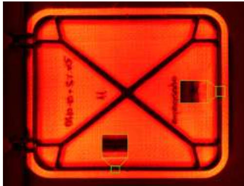
Figure 4: Lack of material close-up look. Punctures undetectable standalone by the human eye
