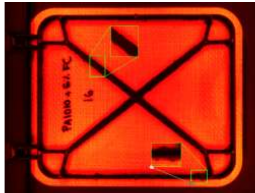
Figure 7: Over-pressure defect close-up, subtle overflowed material around the structural nerves
