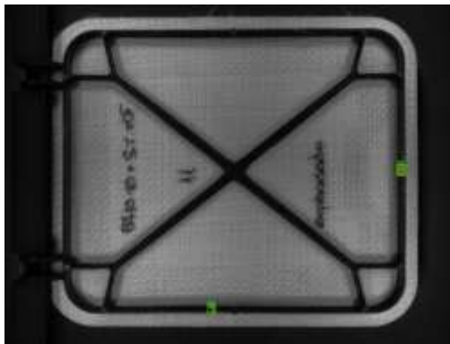
Figure 5: Lack of materials detected by the vision system
